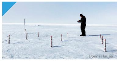
On ice measurements Responding to recent sea ice thinning, Ikaaġvik Sikukun measures sea ice growth and melt over the winter and spring, and tracks snow depth, which insulates the ice keeping it warmer in winter (less sea ice growth) and cooler in spring (less ice melt).
